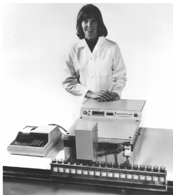
Figure 1.1 The first purpose-built mid-IR analyser based on optical filters manufactured by Foss Electric – MilkoScan 203/300.
